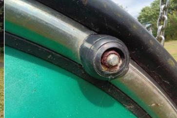
Finding: The fixings have corroded excessively Action: Replace all corroded fixings
